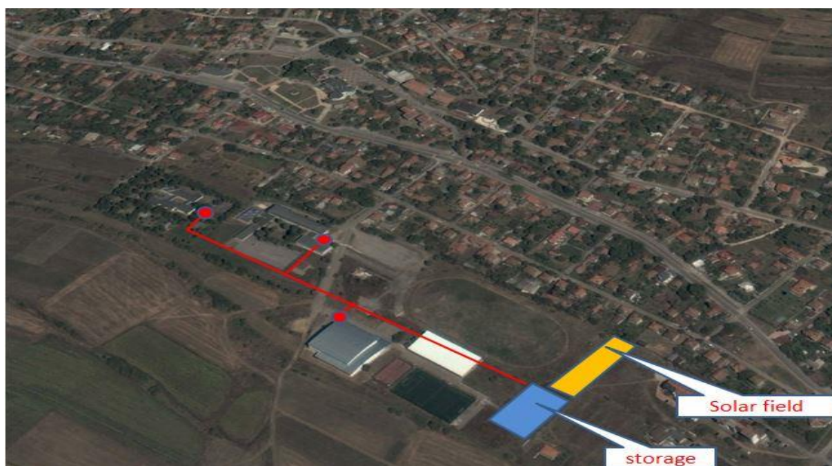
Diagram 1. Phase 1 in the construction of solar district heating in Gorna Malina
