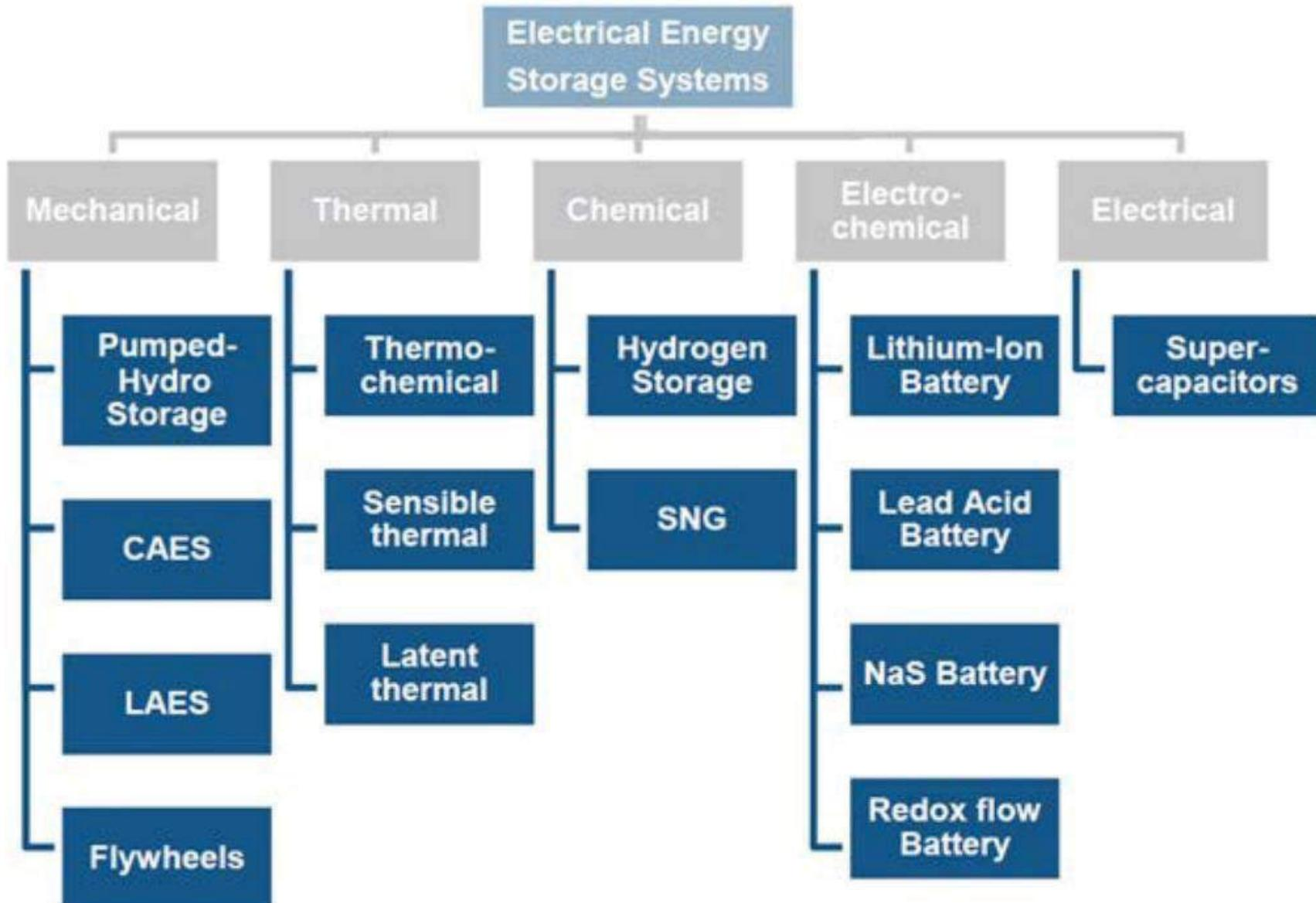
CAES = Compressed Air Energy Storage; LAES = Liquid Air Energy Storage; SNG = Synthetic Natural Gas.
