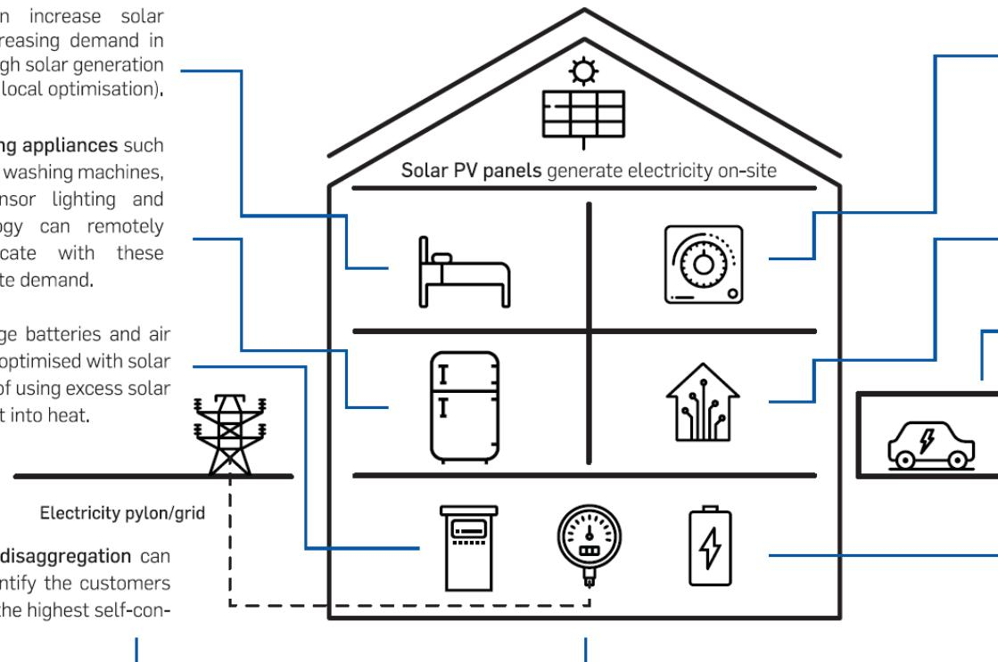
Smart learning thermostats that are internet connected can be combined with electric heating or cooling. Solar providers in the US are already offering customers free smart thermostats.
