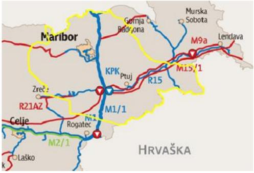
The picture is showing the natural pipeline grid in the Podravje region. With blue colour are marked the existing pipelines and with the red colour the planned pipelines.
